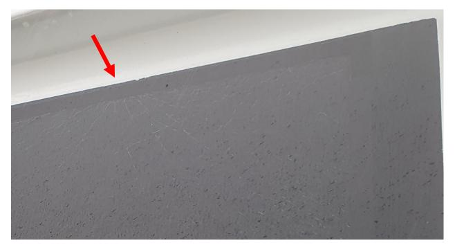
It is clear that the initial fracture was from the top edge, and all the remaining fractures propagate out from there.
