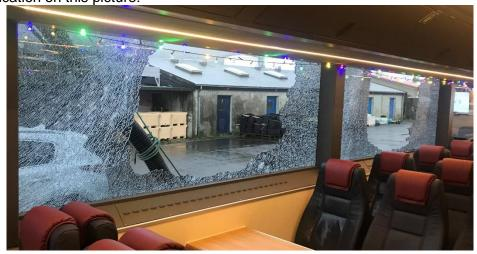
It is also a well know, although quite rare, phenomenon that tempered glass can spontaneously shatter. This happens when a Nickel Sulphide molecule is embedded in the glass. The molecule will be trapped in the glass in a contracted state. Some glass manufacturers use a "Heat Soak Test" to check for this fault. The glass is
